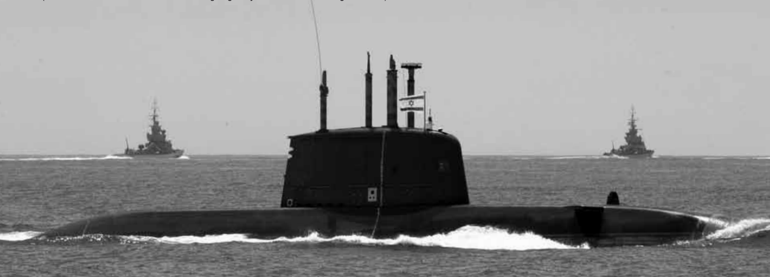
An Israeli Dolphin class diesel electric submarine. The Israelis have huge transit distances to travel to get from the Mediterranean to the Red Sea given the need to avoid the Suez Canal (which must be transited on the surface thus giving away the submarines ‘strategic location’).
