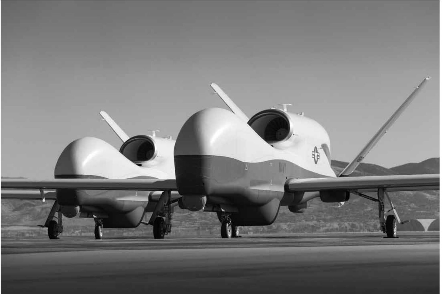
Two USN MQ-4C Triton long range unmanned aerial vehicles. Tritons will be based in the Pacific for the long range persistent intelligence, surveillance and reconnaissance role. (USN)
