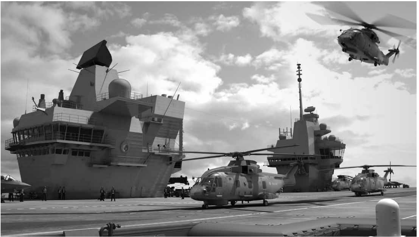
A computer generated image of the unique two island superstructure of the CVFs as well as showing how much room there is on the light deck. (Aircraft Carrier Alliance)
