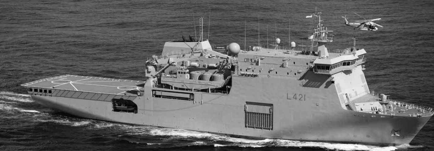
The amphibious warfare ship HMNZS CANTERBURY with Super Seasprite helicopter passing port side. Capable of transporting 296 troops and their equipment and vehicles she can also embark up to four NH-90 helicopters and two landing craft. (RNZN)
