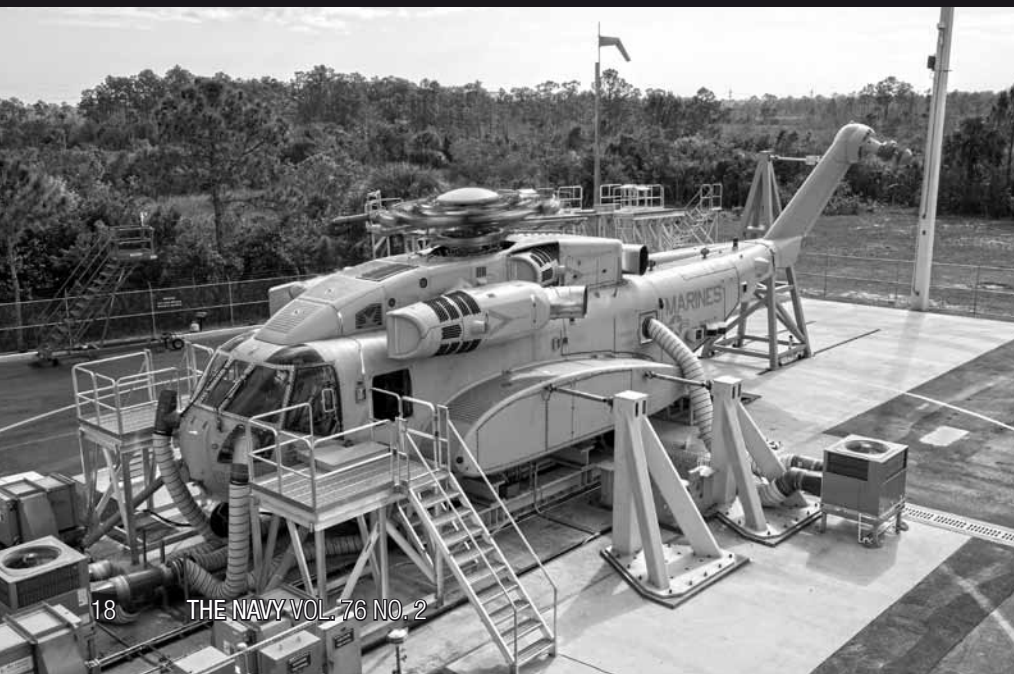
06 Sikorsky's CH-53K heavy lift helicopter Ground Test Vehicle (GTV) undergoing testing. (Sikorsky)
