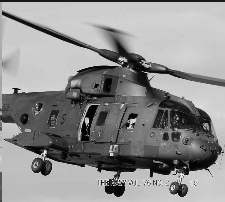
02 An RAF AW101 Merlin helicopter. 25 of these three engined transport helicopters will replace the RN's Sea King Commando helicopters. (RAF)
