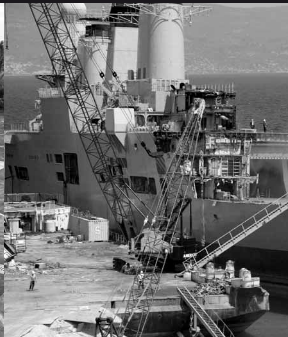
07 The former Invincible class aircraft carrier HMS ARK ROYAL being pulled apart for scrap at a Turkish scrap yard.
