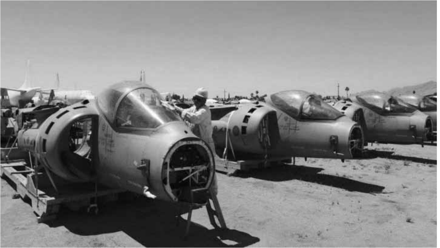
Nearly all of the RAF's GR-9 Harriers were sold to the USMC for spares. Seen here are the remains of the stripped out aircraft now stored in the US desert storage facility at Davis-Monthan Air Force Base Arizona. Keeping the Harriers would have enabled uninterrupted training and experience on STOVL fast jet operations for the CVP's introduction to service. (USAF)
