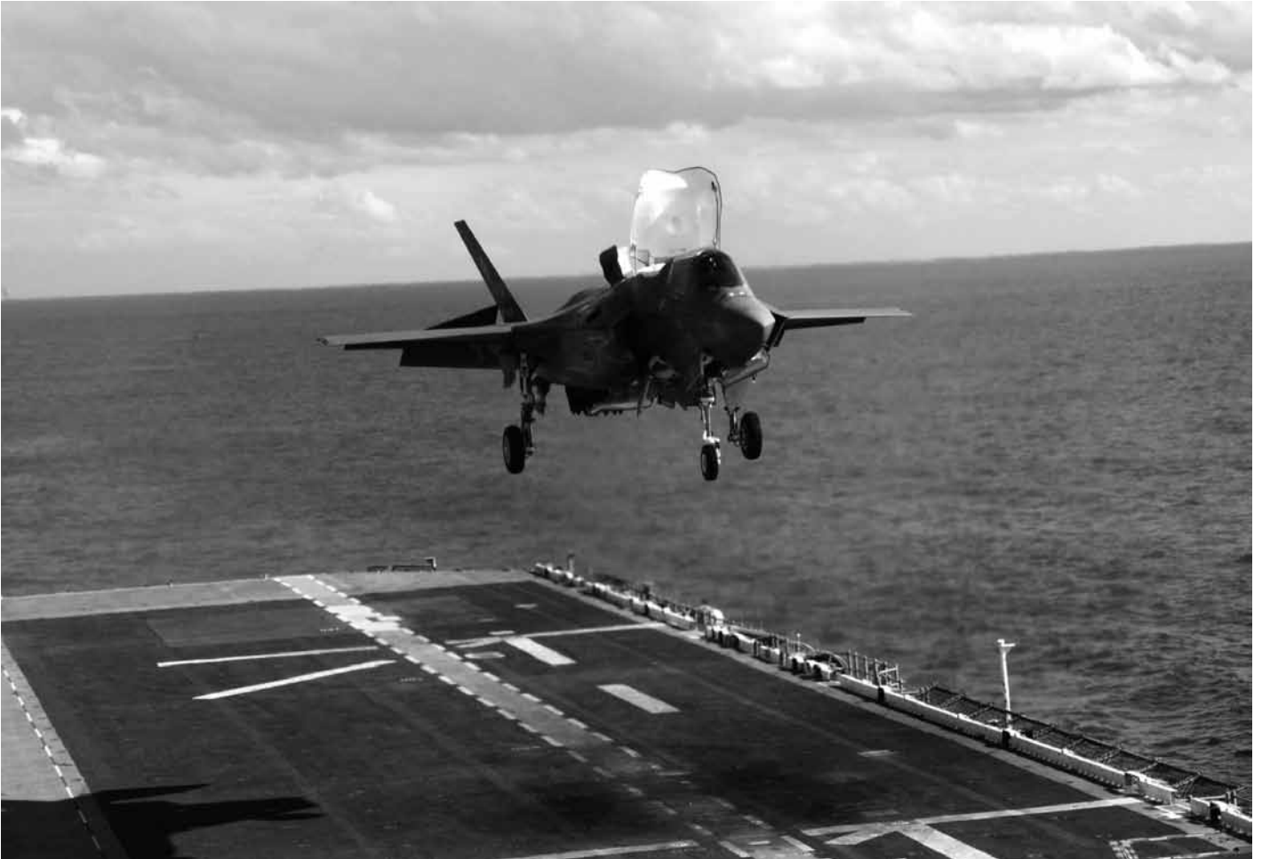
A USMC F-35B STOVL JSF landing aboard USS WASP during first of class sea trials last year. The UK's CVFs were designed to take the F-35B STOVL version of the JSF, then F-35C catapult and arrestor version then changed back again to the B model JSF, at great cost. (USN)
